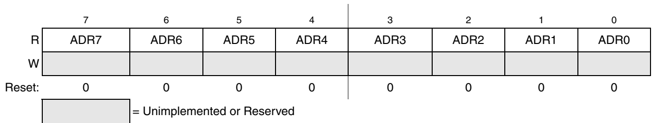
Figure 12-7. Data Result Low Register (ADCRL)
