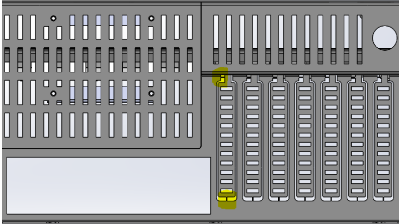
Figure 12 – PCI cutout Knockout example.
